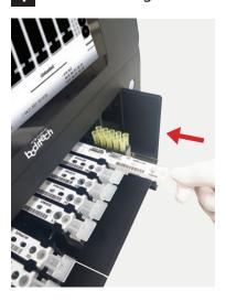
2 Insert sample tube into tube rack
